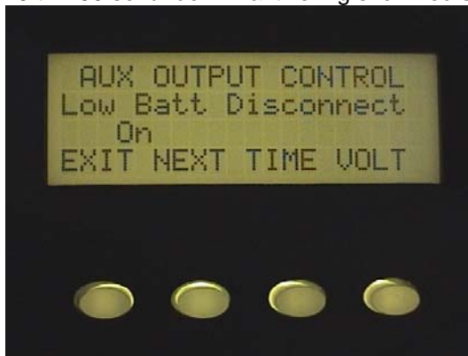
Low voltage disconnect.
