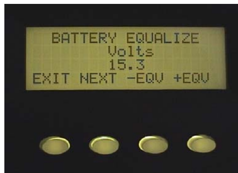
Battery Equalization Voltage Set-up Screen
