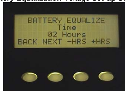
Battery Equalization Time Set-up Screen
