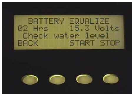
Battery Equalization Start Screen
